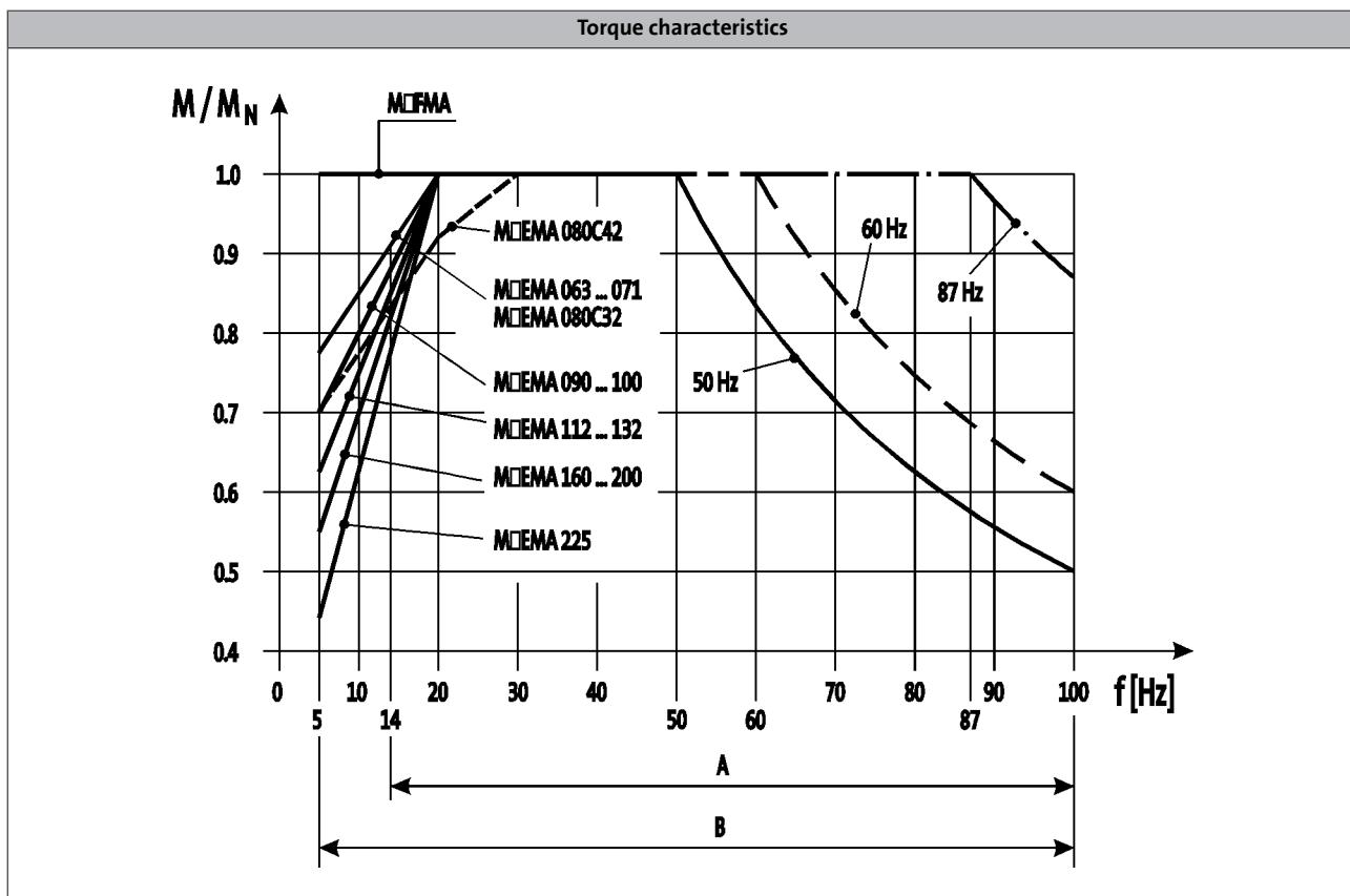
A = Operation with integral fan and brake
